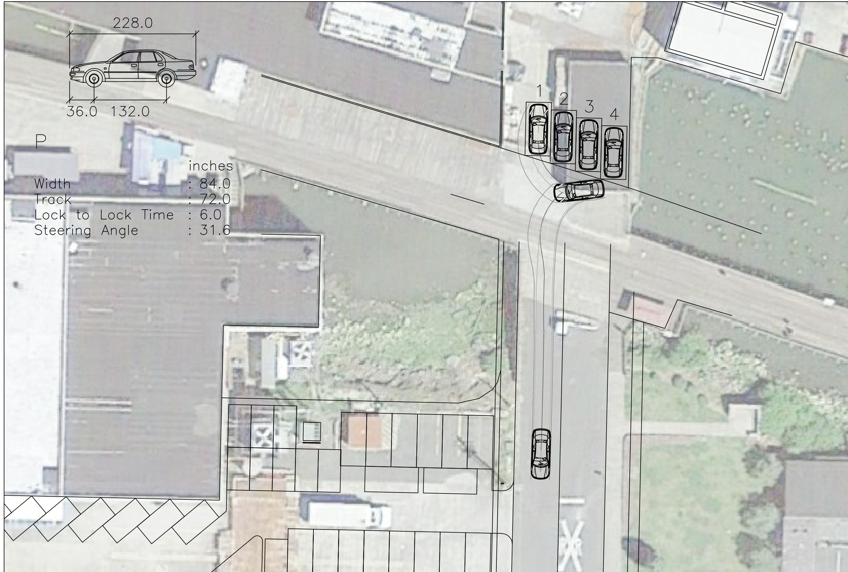
TURNING MOVEMENT ANALYSIS Egress from Parking Stall 1 "P" Design Vehicle
