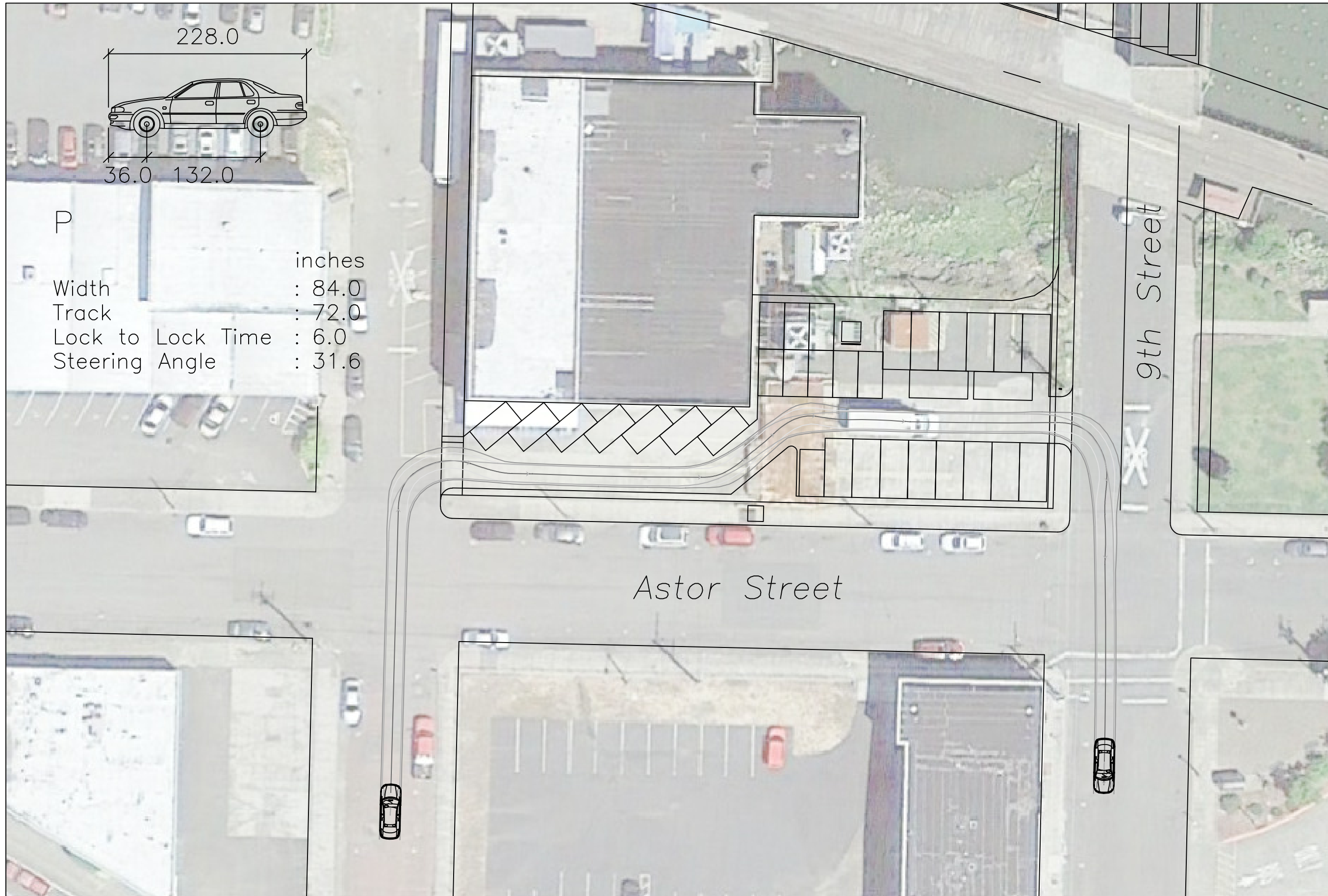
TURNING MOVEMENT ANALYSIS Parking Lot Ingress & Egress "P" Design Vehicle
